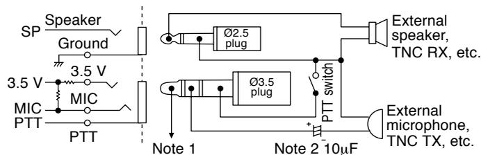
**Note 1:** Voltage is developed across the  $100\ \Omega$  resistor in the 3.5 V line in the transceiver. When 2 mA flows, approximately 3.3 V is developed.
